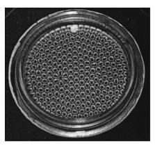
FIG. 8. Imperfections in a hexagonal Bénard convection cell. Aluminum powder shows the motion of a thin layer of silicone oil on a uniformly heated copper plate. The deformity to the left of the pattern is caused by a tiny dent in the plate (Koschmeider, 1974).
